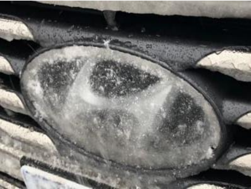
Loss of Sensor
